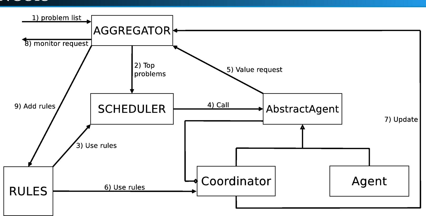
The list of problems reported by the user is filtered and sorted based on the dependencies rules between the services. Each service is then explored in turn, following the exploration order established by the Reinforcement Learning algorithms. Once a faulty
