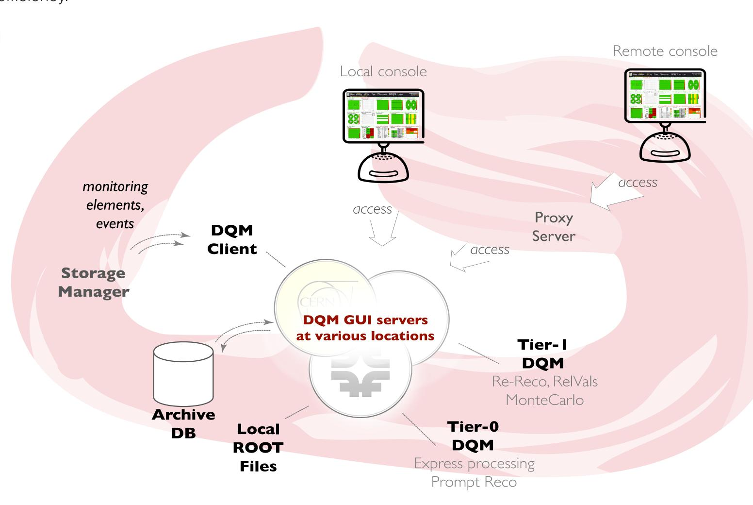
The online DQM applications are an integral part of the rest of the event data processing at the cluster at CMS Point-5. They receive event data and trigger histograms at the rate of about 10-15 Hz. Each application receives events from the storage manager proxy over HTTP and runs its choice of algorithms and analysis modules and generates its results in the form of monitoring elements and including reference histograms and quality test results.
