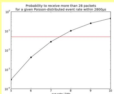
Diagram of example case: A transitory event burst at 10kHz (100µs per event) will saturate the lowest switch after 28 events (2.8ms). The Poisson probability to reach this case becomes significant for a nominal random rate of 7.5kHz (crossing of the 5% dead time limit).
