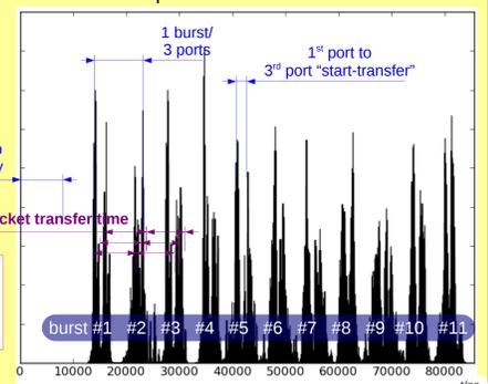
The figure shows the timing pattern of the "start transfer" flags (of physical IP traffic), measured for 11 bursts of 1kB-packets (broadcast time 8µs over 1Gbps) sent out over three ports each.
