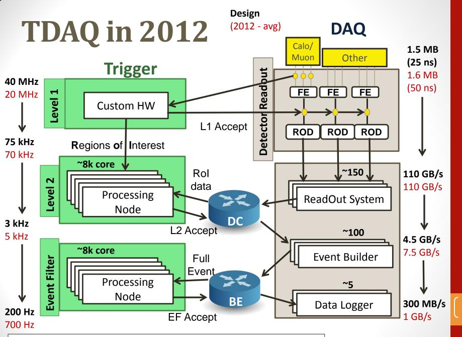
*Note*: Level 2 (L2) + Event Filter (EF) = High Level Trigger (HLT)
