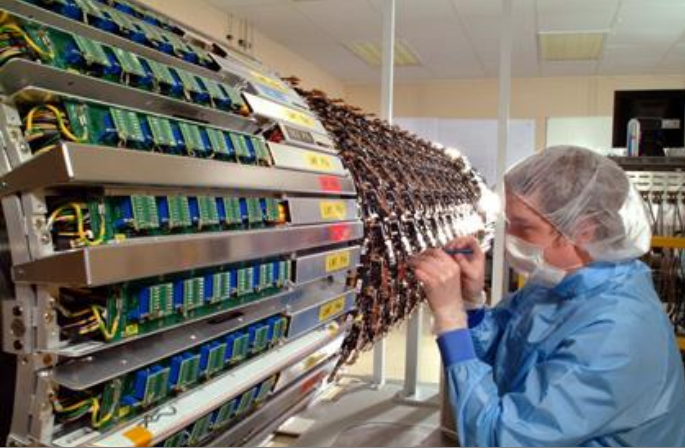
ATLAS Barrel Semi-Conductor Tracker (SCT) Engineering, Design, Project Management, Service assembly at RAL
