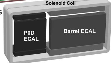
Electromagnetic calorimeters provide EM energy measurement and additional particle identification
