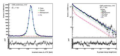
2011 result from CMS-PAS-BPH-11-006: time-dependent angular analysis Plots correspond to projections of a five-dimensional likelihood  $c\tau(B_5^0) = 0.04580 \pm 0.00059 \text{ (stat)} \pm 0.00022 \text{ (syst) cm}$
