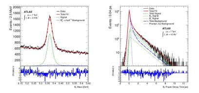
2011 result from JHEP 12 (2012) 072: time-dependent angular analysis Plots correspond to projections of a five-dimensional likelihood  $\Gamma_s=0.677\pm0.007~(\text{stat})\pm0.004~(\text{syst})~\text{ps}^{-1}$
