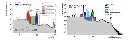
Both experiments implemented trigger selections specific to *B*-physics studies, to complement single and double muon triggers (both plots based on 2011 data)
