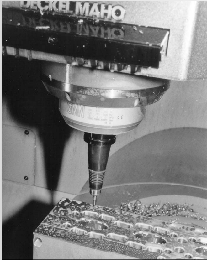
Direct 5-axis milling of cooling water circuit groove in PEP-II cavity.
