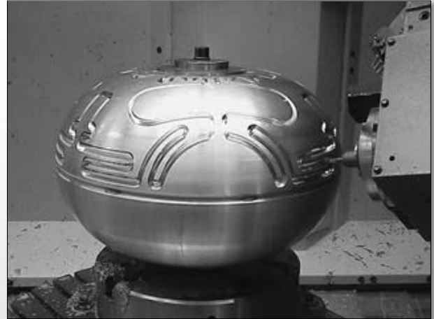
Direct 5-axis milling of cooling water circuit groove in PEP-II cavity.
