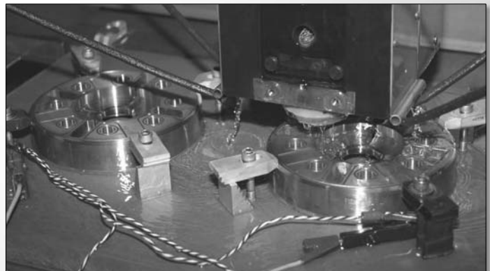
wire cutting of the iris slots of SICA (slotted iris – constant aperture) disks for CERN's CTF3 drive beam accelerator
