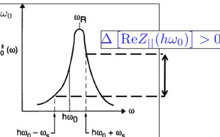
**Figure 4.4.** Illustration of the Robinson stability criterion. The rf fundamental mode is detuned so that  $\omega_r$  is (a) slightly below  $h\omega_0$  and (b) slightly above  $h\omega_0$ . (a) is Robinson damped above transition and antidamped below transition. (b) is antidamped above transition and damped below transition.
