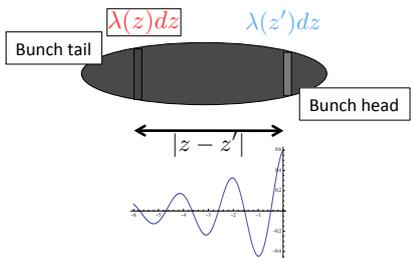
$$\underbrace{\frac{d^2z}{dt^2} + \frac{\eta e V_{\text{rf}}(z)}{m_0 \gamma C}}_{\text{External RF}} = \underbrace{\frac{\eta e^2}{m_0 \gamma C} \sum_{k=-\infty}^{\infty} \int_{-\infty}^{\infty} \lambda(z' + kC) W_{||}(z - z' - kC) dz'}_{\text{Wake fields}}$$
