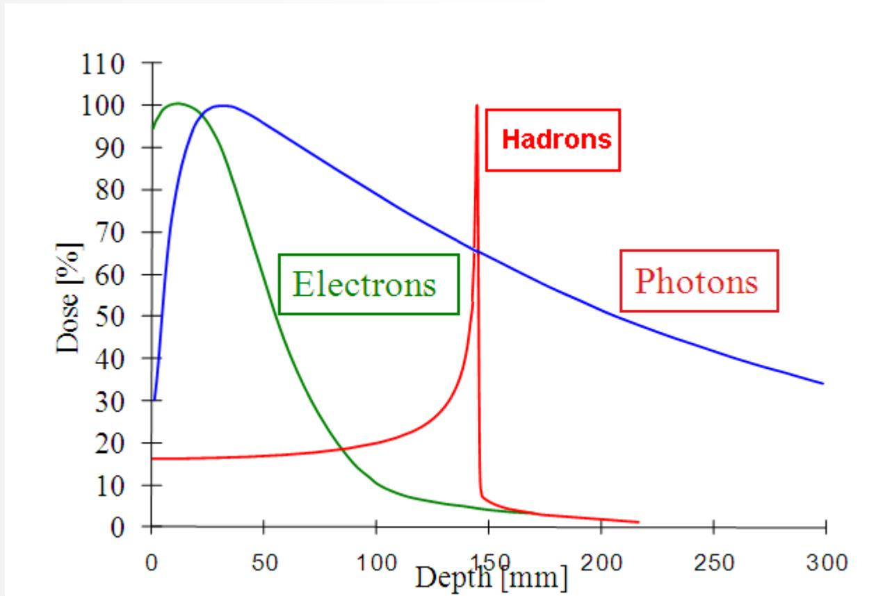
The depth and magnitude of the Bragg peak is determined by the mass and charge, as well as the particle initial energy
