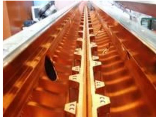
Medium frequency (176 MHz), high duty cycle (CW), 4-rod design for high-intensity deuteron and proton acceleration.
