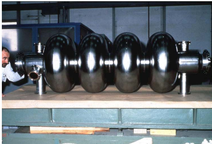
Superconducting LEP cavity
