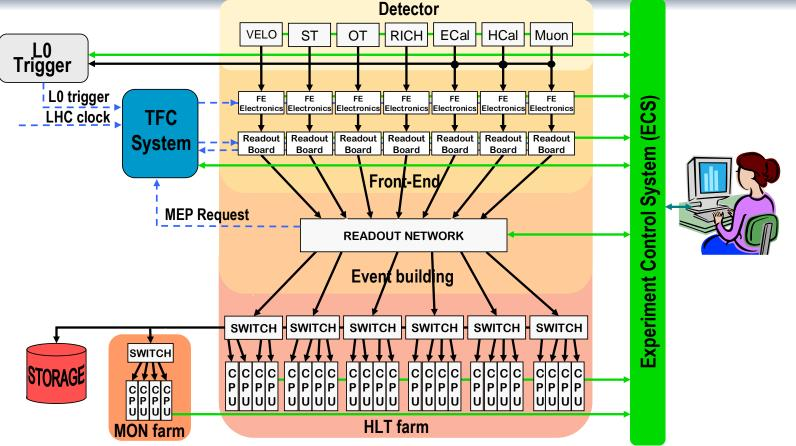
Event data Timing and Fast Control Signals Control and Monitoring data
