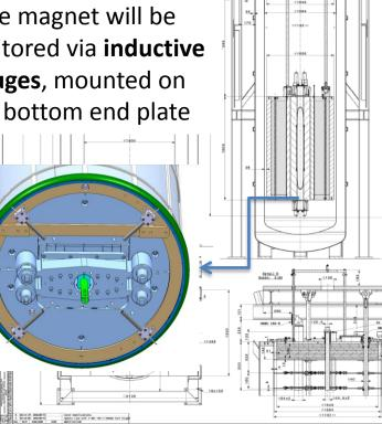
In order to be **flexible** during the magnet insertion in the cryostat, the top-plate is free to move by **2 cm** in its transverse plane.
