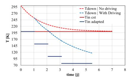
The temperature at the bottom of the magnet
