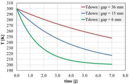
With 36 mm gap the cooling to 180 K would take about 20 days while with 6 mm, 5 days. From this moment  $LN_2$  can be used and in less than 1 day, everywhere in the structure, the 77 K will be achieved. Then the filling of about 1000 I of  $LN_2$  will take an additional day.
