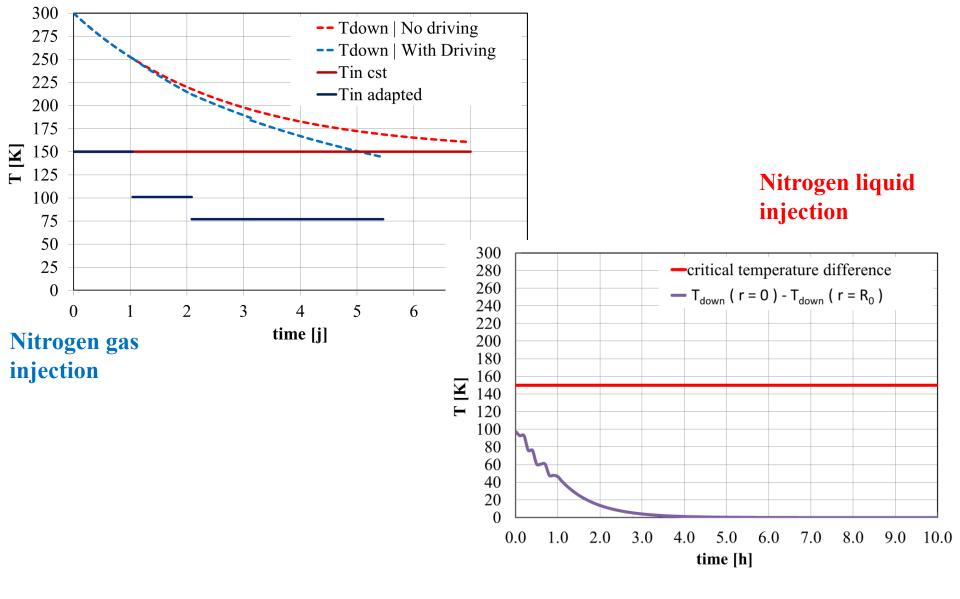
In case 150 K difference is allowed with a 10mm gap, we inject the 1<sup>st</sup> day gas at  $T_{in} = 150$  K then the 2<sup>nd</sup> day at  $T_{in} = 100$  K, the 3<sup>rd</sup> day liquid can be injected safely. In 4 days, the magnet is cold.
