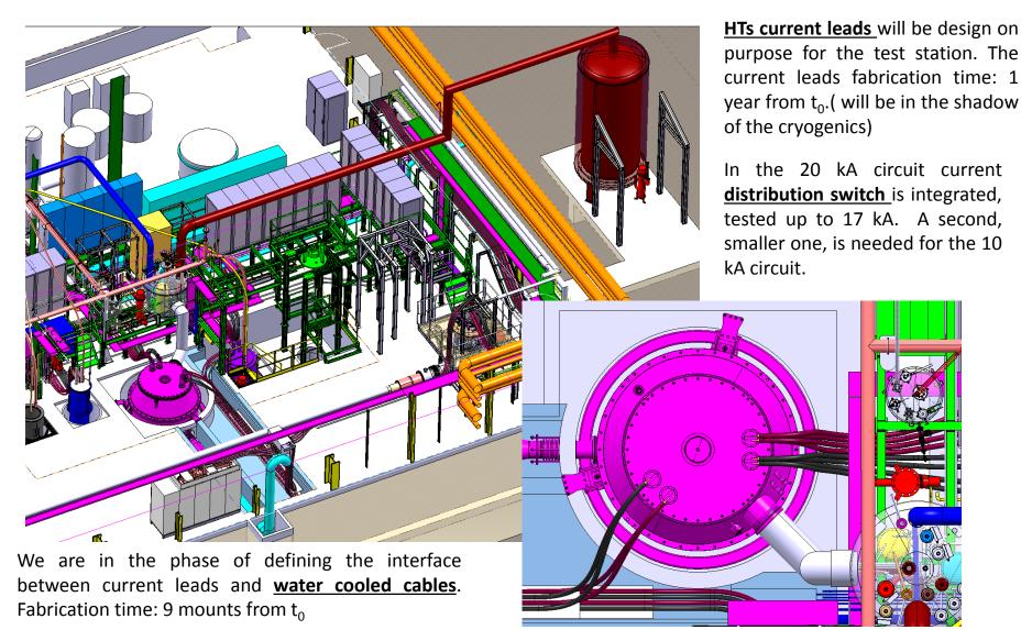
8 x 500 mm copper water cooled cables between bus bars and current leads for the 20 kA circuit 4 x 500 mm Cu water cooled cables between 10 kA power converter and inserts trough a dedicated switch ( < than the existing 16 kA)
