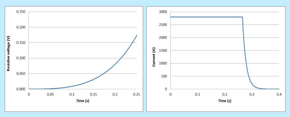
Resistive voltage and current decay of the insert "alone" during a fast discharge for quench
