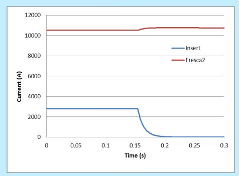
If Fresca does not quench for the current bump, the current decay follows Fresca constant time  $\tau = 1.3$  s 1 - Quench with fast discharge for the insert <u>without</u> a discharge for the Fresca dipole (continued)
