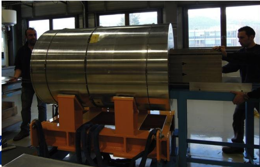
The pre-assembled yoke and shell are rotated to horizontal position
