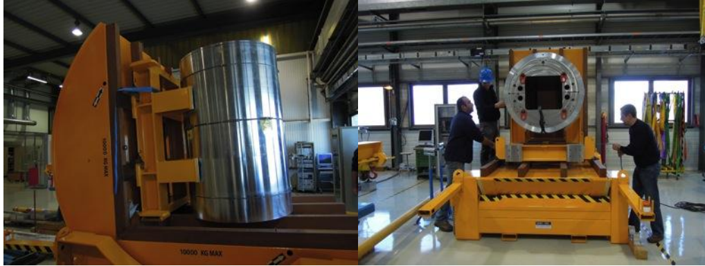
The pre-assembled yoke and shell are rotated to horizontal position
