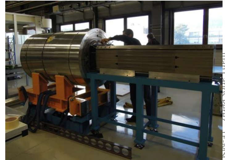
Magnet structure installed on the assembly table
