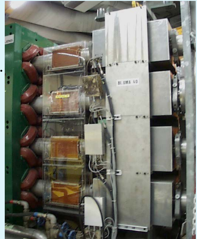
The 4 rings of the CERN PS Booster
