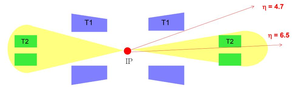
**Event selection:** Trigger with T2, at least one track in <u>both</u> T2 hemispheres, <u>no tracks in T1</u> "(0T1+2T2) topology".
