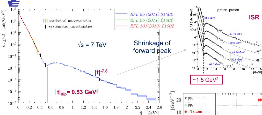
$d\sigma/dt \sim e^{-B|t|}$  Increase of B slope with collision energy
