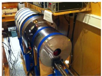
2G 755-R SQUID Cryogenic rock long core rock magnetometer ETH, Zurich Nominal sensitivity  $<< g_D$
