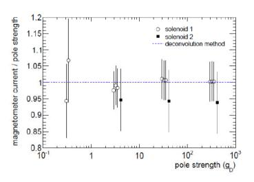
Flat behaviour once solenoid is extended into the sensing region Linear and charge symmetric 5-6% differences between solenoids. Nominal sensitivity to  $\sim 0.32g_D$
