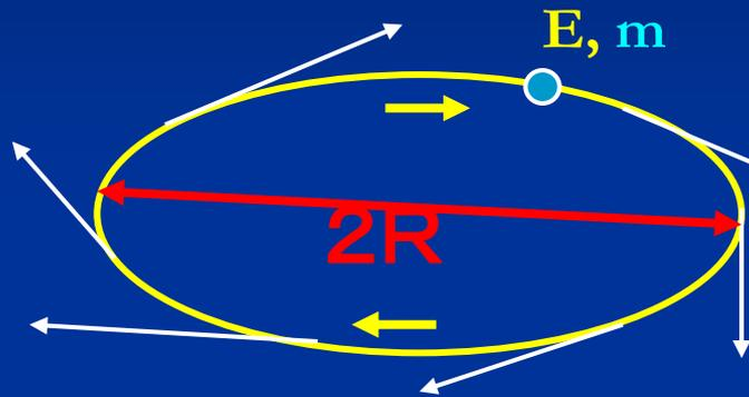
Electron and positrons lose energy due to synchrotron radiation
