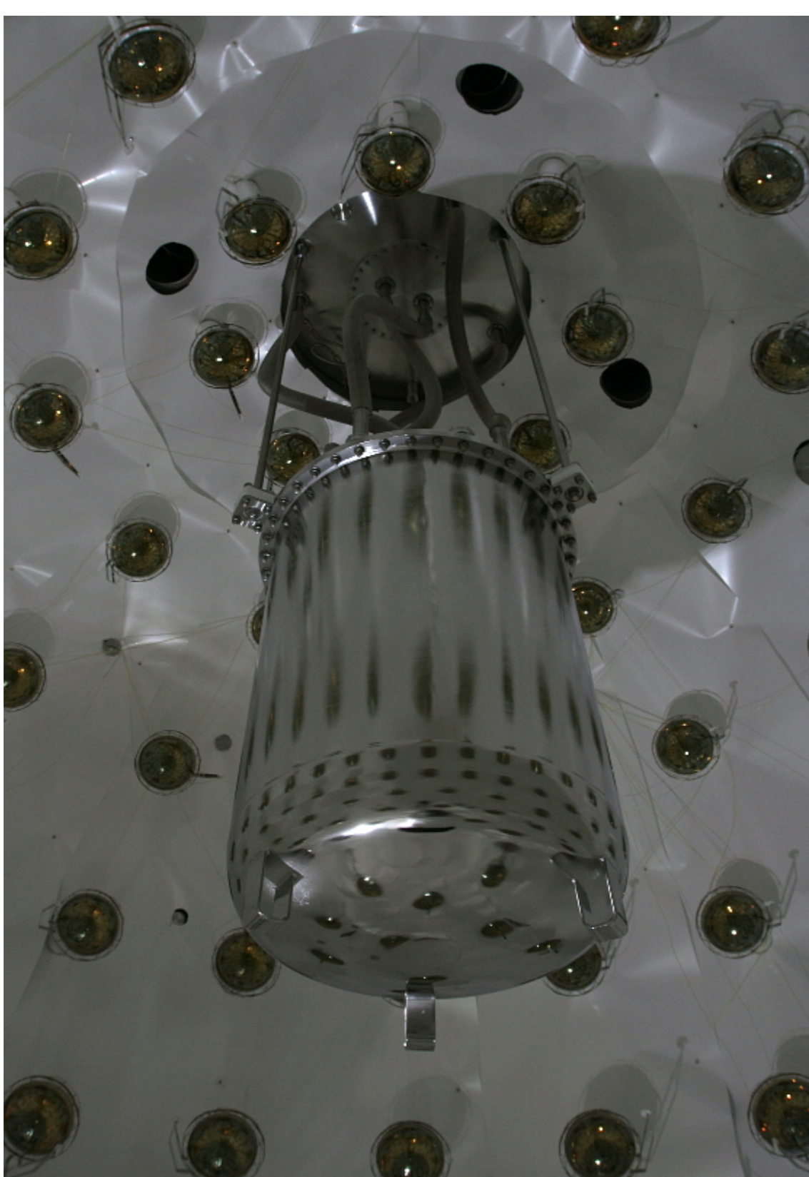
Fig. 3 The DS-50 TPC inside the Neutron detector.
