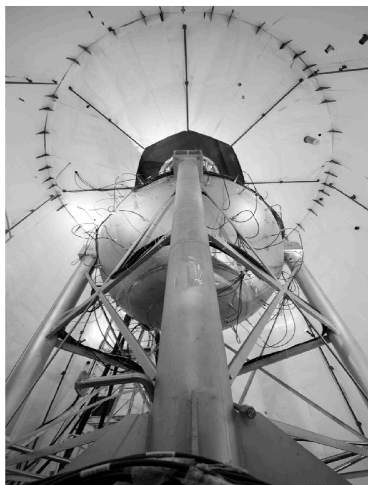
Fig. 4 The Neutron detector inside the CTF.
