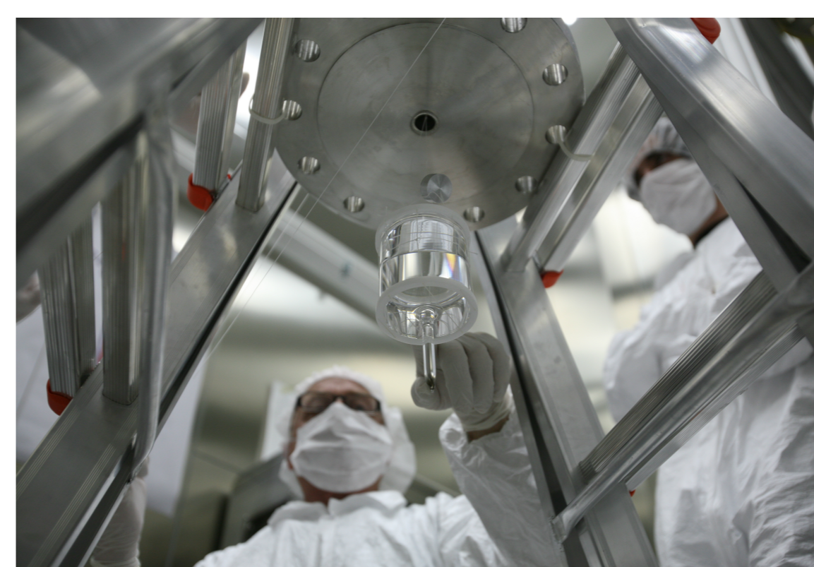
Fig. 6 The PC cell and the ^{241}\text{Am} before the insertion.
