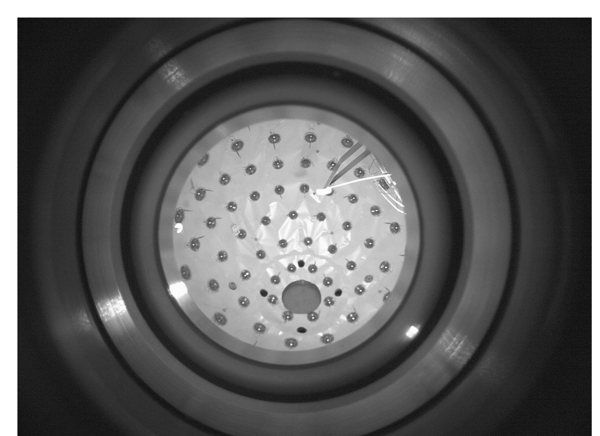
Fig. 7 The PC cell and the ^{241}\text{Am} inside the neutron detector.
