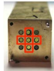
CFCAL is a brass absorber with 9 LuAG fibers
