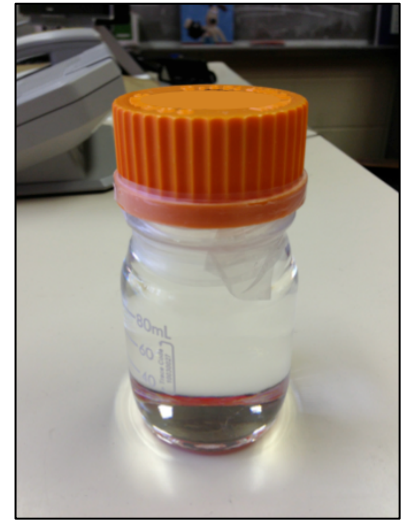
Optically transparent Te-loaded scintillator
