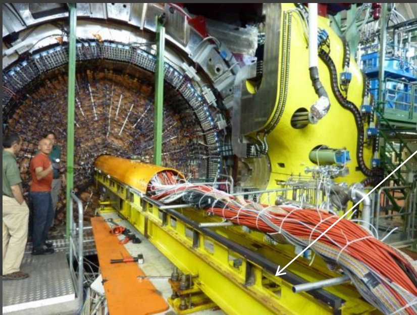
Rails to support and insert IR
