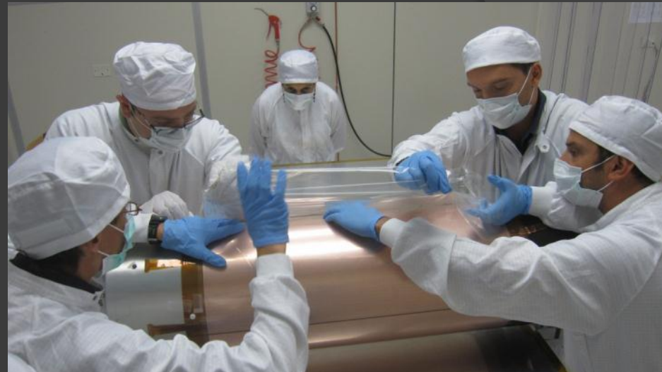
GEM is wrapped on a cylindrical mold
