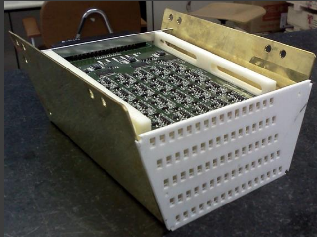
FEE with HV regulator, preamplifier and splitter
