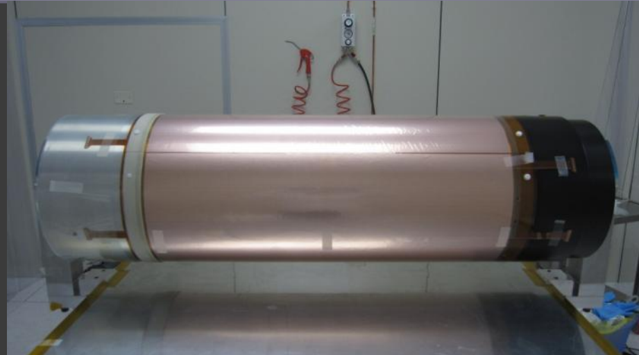
Final cylindrical GEM with internal and external rings
