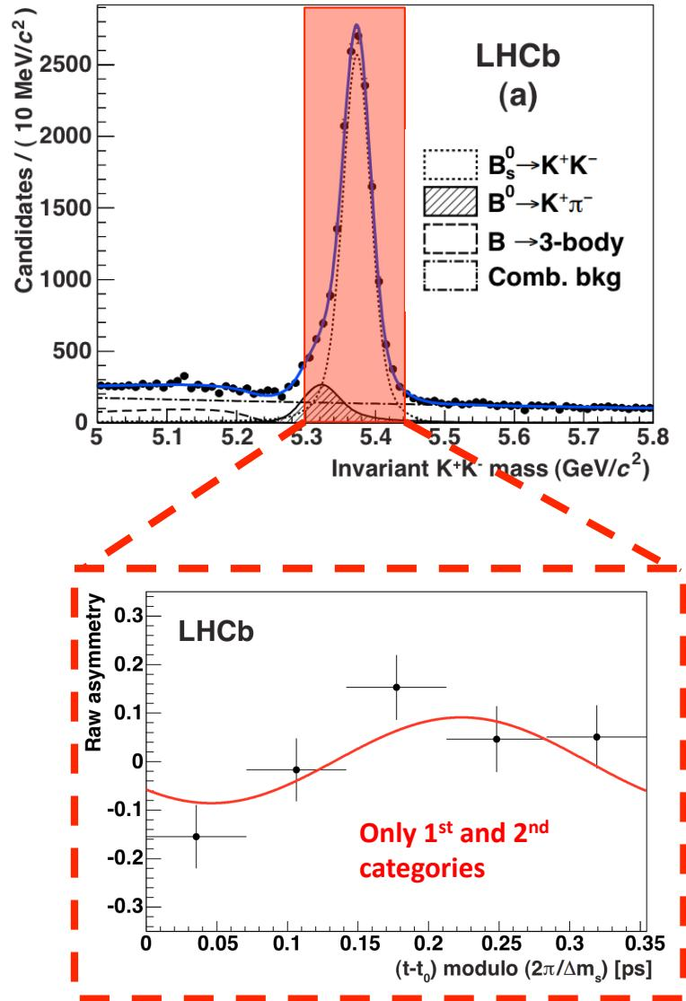
$$\mathcal{A}(t) = \frac{-C_f \cos(\Delta m_s t) + S_f \cos(\Delta m_s t)}{\cosh\left(\frac{\Delta\Gamma_s}{2}t\right) - A_f^{\Delta\Gamma} \sinh\left(\frac{\Delta\Gamma_s}{2}t\right)}$$
