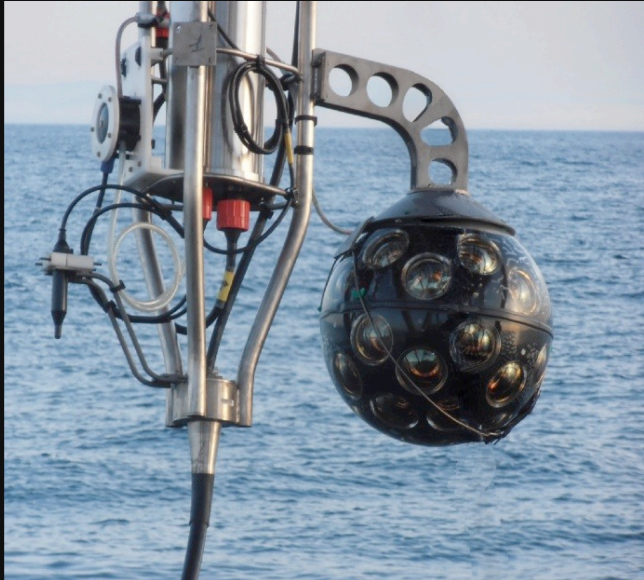
test installation on ANTARES instrumentation string
