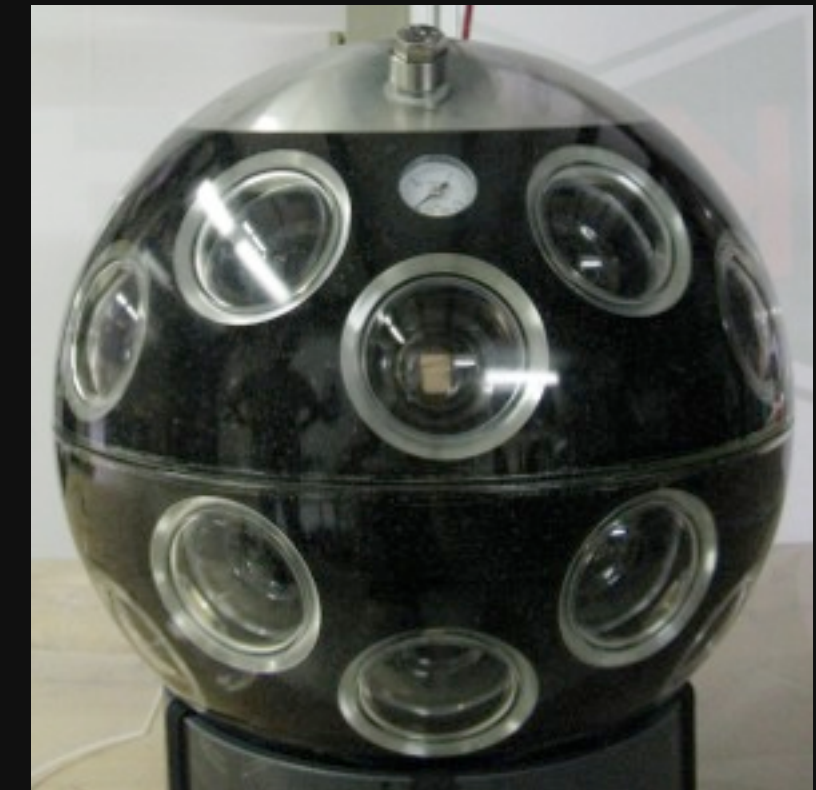
Multi-PMT digital optical module (“DOM”)
