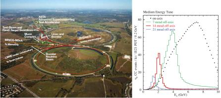
Medium energy tune, 7 GeV peak on-axis, 2 GeV peak 14.6 mrad off-axis to Ash River
