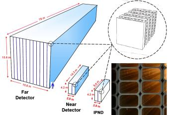
14 kt, 65% active far detector, 15.6 m plastic cells filled with liquid scintillator, each plane just 0.15  $X_0$ .
