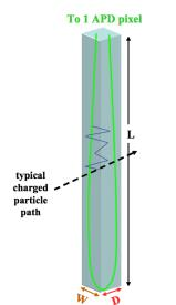
Each cell readout by a looped wavelength shifting fibre connected to an avalanche photodiode.
