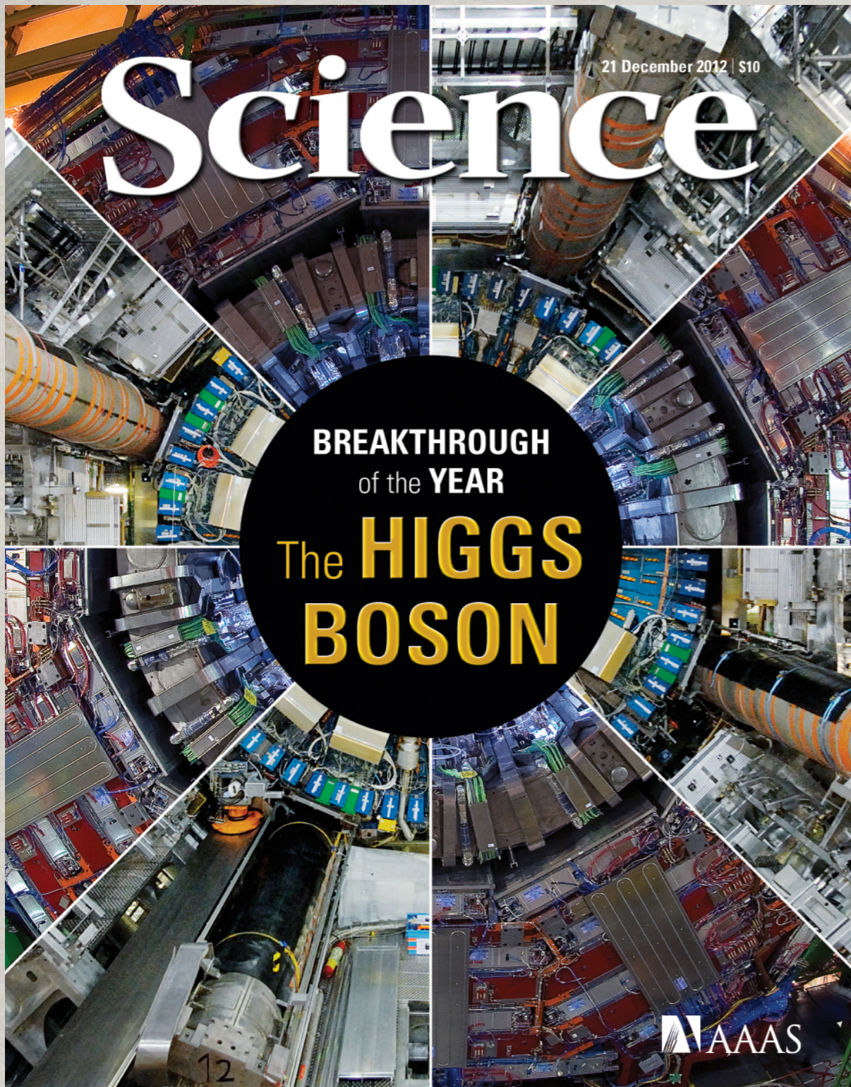
Mosaic of the CMS and ATLAS detectors (as in 2007), part of the Large Hadron Collider at CERN. In 2012, research teams used these detectors to fingerprint decay products from the long-sought Higgs boson and determine its mass, successfully testing a key prediction of the standard model of particle physics.
