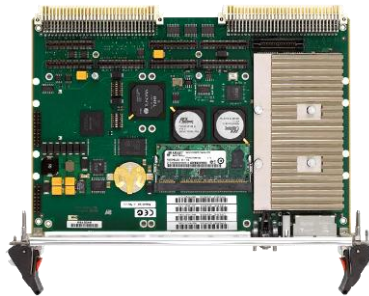
VME Card: Eurocard size VMEbus interface
