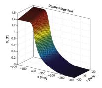
Dipole fringe field. Quadrupole and sextupole field components can be seen by looking at the transverse slope and curvature, respectively.
