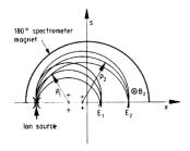
Mass spectrometer: particles are separated according to their energy and focused due to the  $1/\rho$  effect of the dipole
