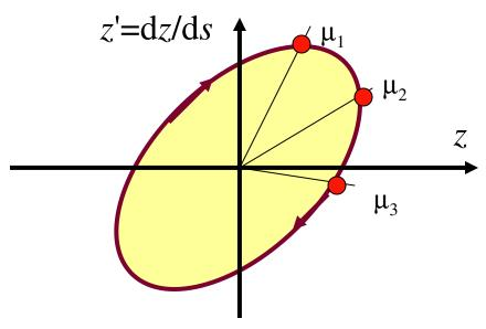
★ In the case of a ring or matched cell, the periodicity imposes equality on the input and output α and β values. This means that the particle returns after each turn or transit to the same ellipse but at phases  $\mu_1=B$ ,  $\mu_2=B+2\pi Q$ ,  $\mu_3=B+2\pi Q$ , ....,  $B+n2\pi Q$  and so on.
