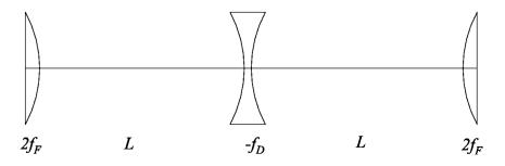
This exercise considers a general case where  $f_F$  is not necessarily equal to  $f_D$ . Using the thin lens approximation for the FODO cell with drifts of length L we get the following matrix:
