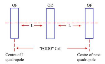
Show that the transfer matrix of a FODO system in thin lens approximation is as follows:
