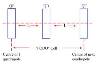
Show that the transfer matrix of a FODO system in thin lens approximation is as follows:
