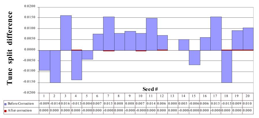
Local decoupling using 16 skew quadrupole correctors and coupled response matrix reconstruction
