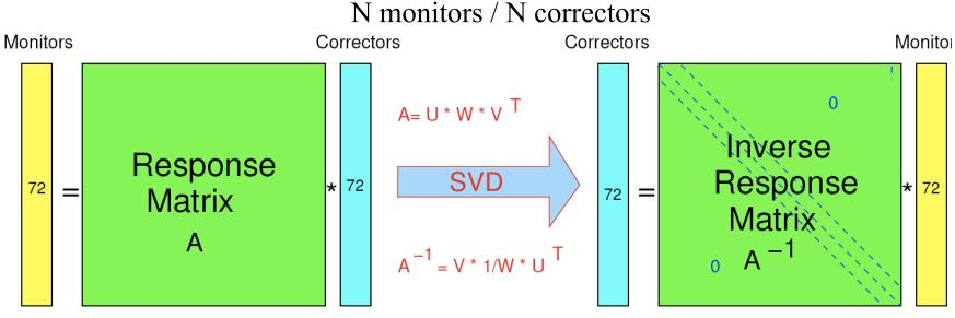
=> Minimization of the RMS orbit (=0 in case of "Matrix Inversion" using all Eigenvalues)
