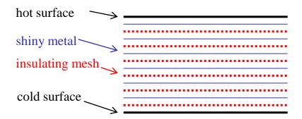
Because radiated power goes as  $\theta^4$  you can reduce it by subdividing the gap between hot and cold surface using alternating layers of shiny metal foil or aluminized Mylar and insulating mesh. Note - the structure must be open for pumping.
