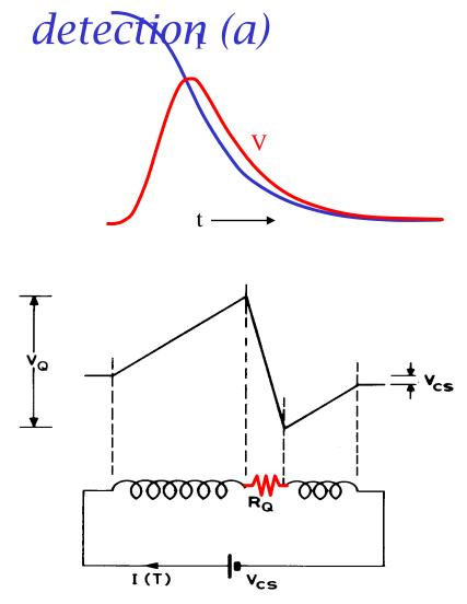
internal voltage  $V = IR_Q = -L\frac{dI}{dt} + V_{cs}$ after quench
