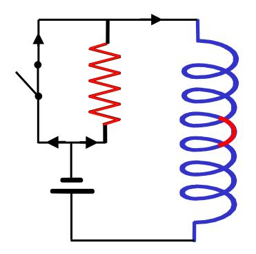
Note: circuit breaker must be able toopen at full current against a voltage $V = I.R_p$
