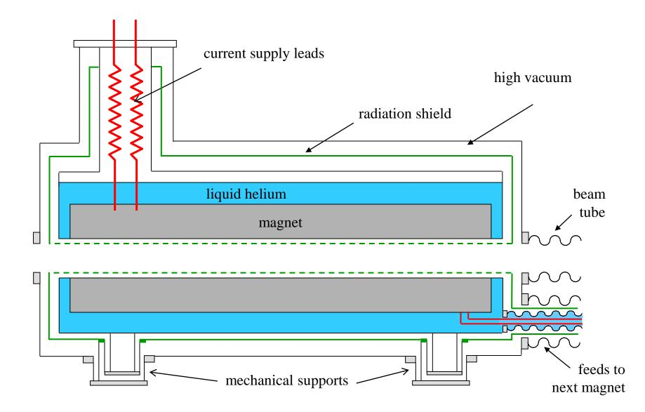
Cryogenic heat leaks
