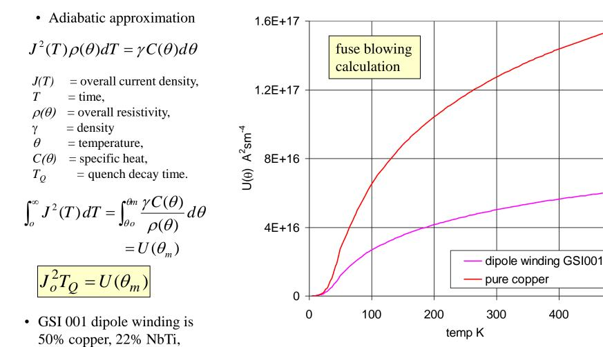
household fuse blows at 15A, area = 0.15mm<sup>2</sup> J = 100Amm<sup>-2</sup> NbTi in 5T J<sub>c</sub> = 2500Amm<sup>-2</sup>
