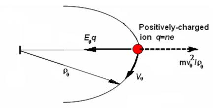
Alternatively, the equivalent of cyclotron motion is found simply by equating the expressions for the centripetal force,
