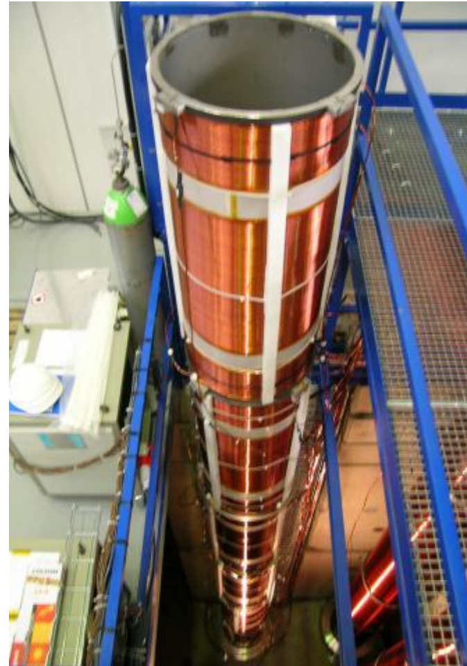
NEG coating unit at CERN
