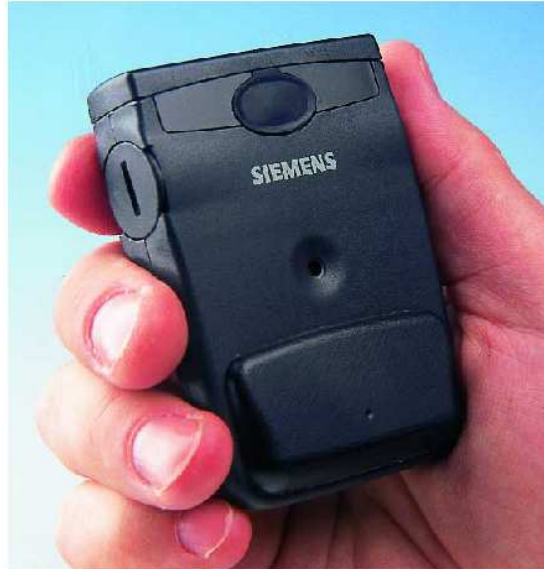
Figure 59 – Picture of the EPD-N photon and neutron electronic dosimeter from the company Siemens [31].
