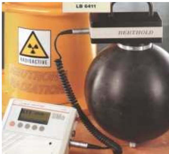
Figure 53 – The EG&G Berthold LB 6411 ambient dose equivalent rate meter
