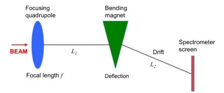
1.1 If the effective length of the dipole is  $l_B=0.43$  m, what should be the magnetic field (in Tesla) inside the dipole to deflect the electrons by an angle of 35 degrees?
