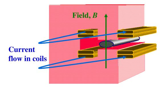
C-shaped' dipole. Useful for injection, extraction and junctions in transfer lines. Often the poles are inclined to superimpose a gradient on the dipole field.
