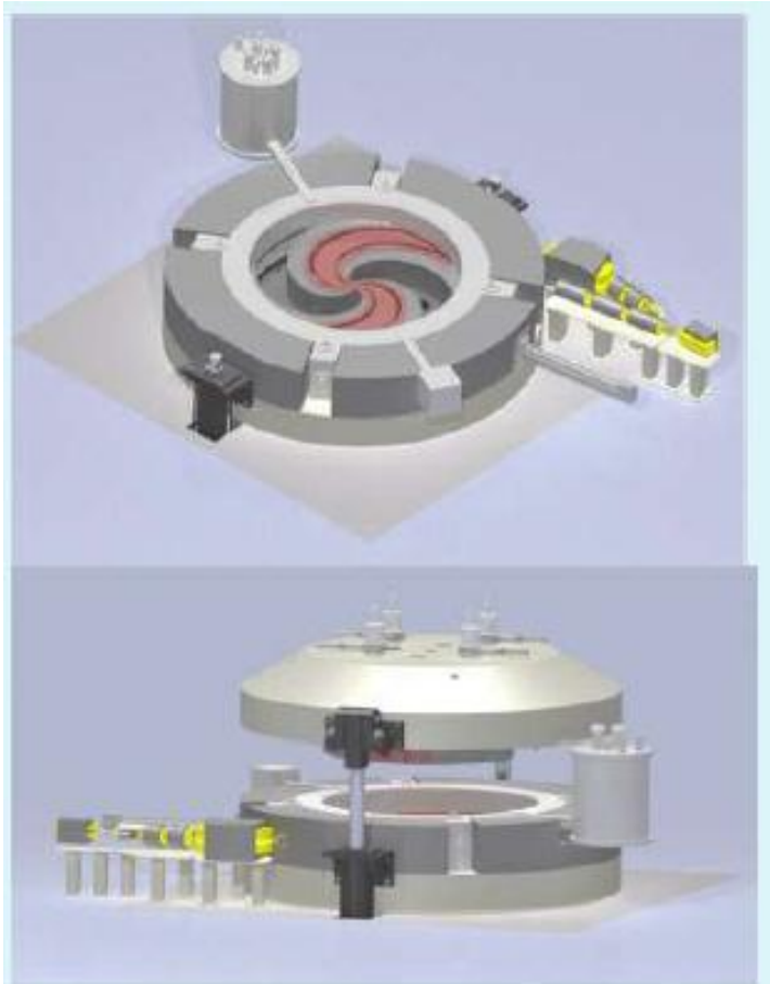
IBA C400 Cyclotron : 400MeV/u carbon , 265 MeV p ( B_c = 4.5 T)
