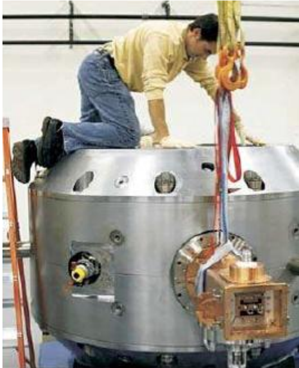
9 T superconducting Synchro-cyclotron
