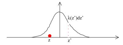
To this end we calculate the effect on the charge from the whole bunch by means of the convolution integral:
