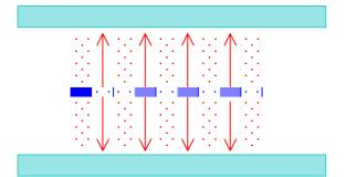
Because of the symmetry, the fields are the same as in the free space. The transverse fields intensity reproduce longitudinally the charge density.
