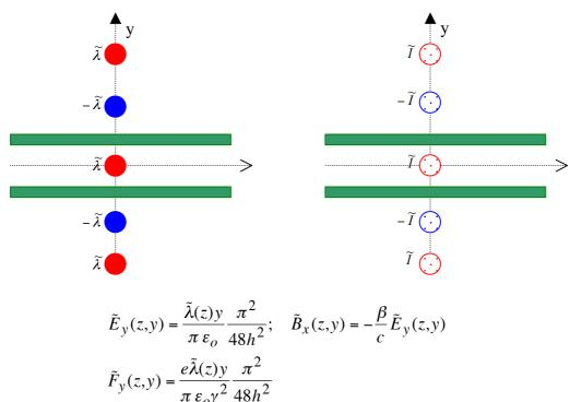
Combining with the direct space charge force, we get for the a.c. component:
