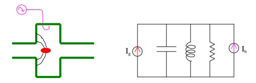
The voltage in the cavity is given by a combined effect of the two currents. We have seen that the beam current is impulsive, and repeats at each beam passage. The generator current feeding the cavity is an alternate signal at the RF frequency:
