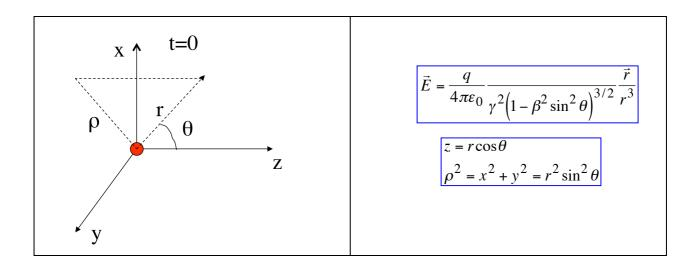
It is easy to see that for  $\theta = \pi/2$ , the radial electric field is proportional to the charge energy, while for  $\theta = 0$ , the electric field vanishes as (energy)<sup>-2</sup>.
