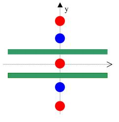
Where we have assumed h >> a > y. For d.c. or slowly varying currents, the boundary condition imposed by the conducting plates does not affect the magnetic field. As a consequence there is no cancellation effect for the fields produced by the "image" charges.
