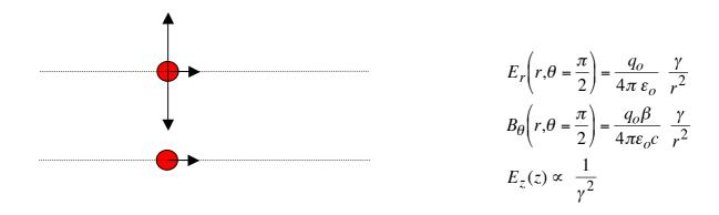
It is interesting to calculate the e.m. forces between two ultra-relativistic charges travelling on parallel trajectories. The longitudinal force is proportional to the electric field  $E_z$ , and vanishes as  $1/\gamma^2$ , while the transverse force vanishes because electric and magnetic fields effects have opposite sign:
