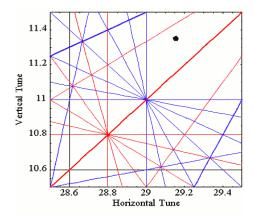
A resonance diagram for the Diamond light source. The lines shown are the resonances and the black dot shows a suitable place where the machine could be operated.
