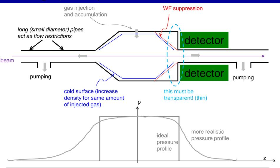
Reminder: contrary to VELO/LHCb, here gas injection must be continuous (with beam)... Consider impact on machine!
