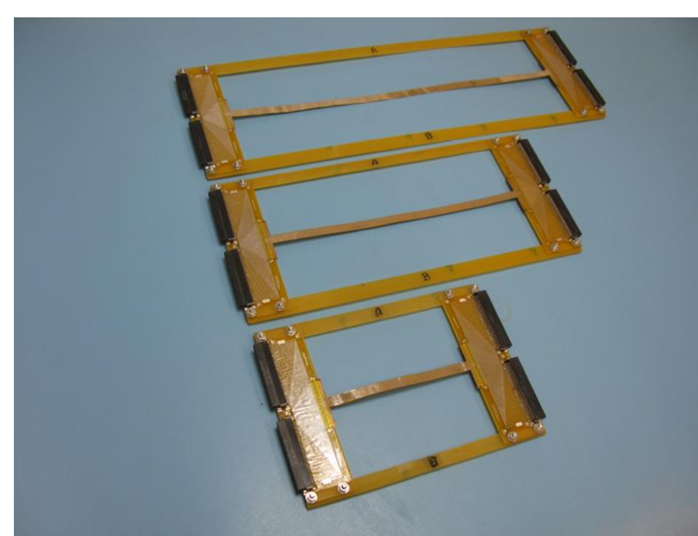
Low-mass micro cables prototypes 10 cm, 20 cm and 30 cm
