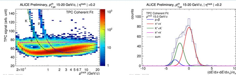
The TPC Coherent Fit extracts the particle composition for a given track sample by fitting both TPC  $dE/dx$  model parameters and particle content at the same time ("coherence") to data.
