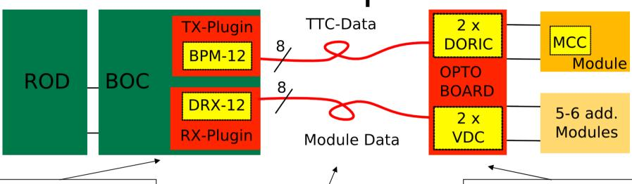
Off-Detector optical components
