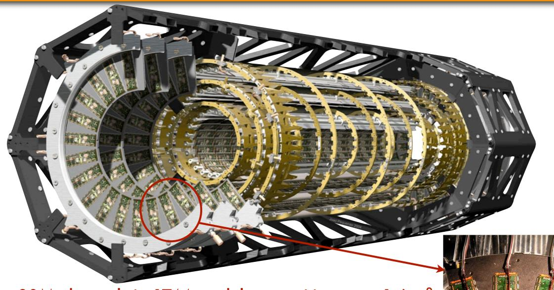
80M channels in 1744 modules, sensitive area 1.6 m<sup>2</sup> Coverage up to  $|\eta| < 2.5$  with 3 points Innermost layer at R=5cm
