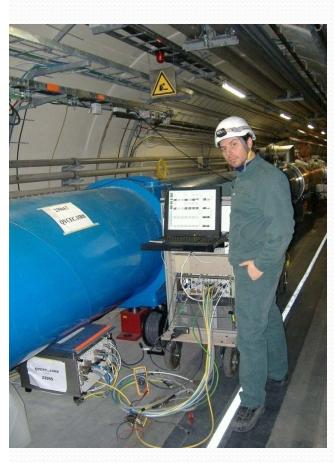
The MTB is based on a PXI platform, running LabVIEW<sup>TM</sup> application. The PXI rack houses:
